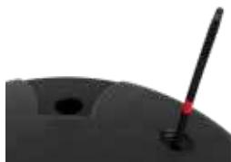
The hole on the lid of the Ejektortank is intended for a Ø32 mm urine hose. On the lid there is also a float indicator tube that shows when the container starts to get full. When the red mark is displayed, another 5 liters remain before it overflows.
